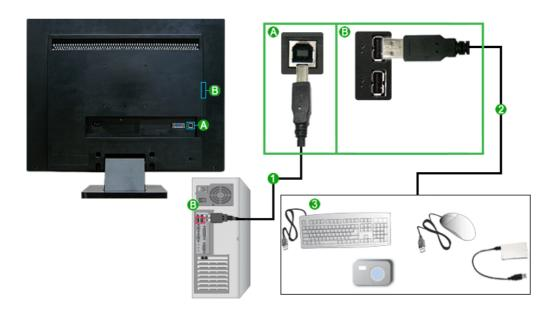
Oconnect the ← Aport of the monitor and the USB port of the computer with the USB cable.
